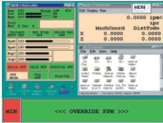
The touch screen operator interface leverages the concept of soft control buttons versus hardware buttons.
