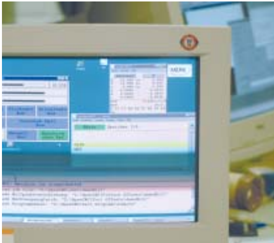
The control commands are sent from the image-processing PC via the OpenCNC PC (at the front) to the measuring machine.
