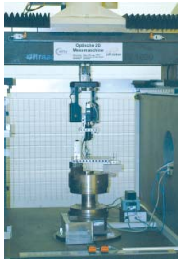
OpenCNC controls the camera via three linear and three rotary axes with a precision of up to five micrometers.
